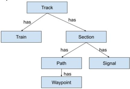
This diagram is meant to show the way in which objects are held. One track has many trains and many sections on it. Each section has a path to follow and two signals at either end. Paths are made up of Waypoints.
